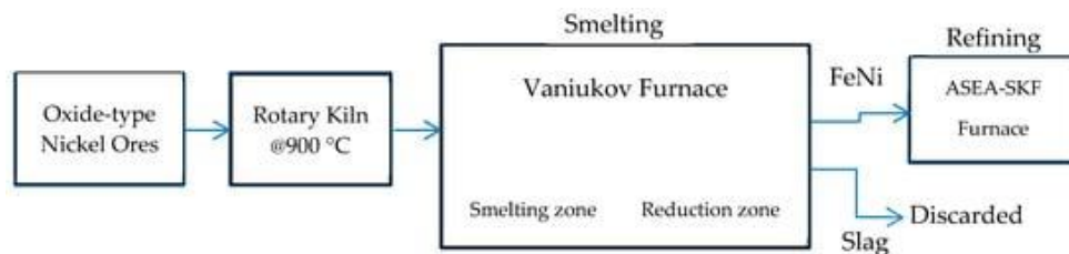
Gambar 2. Proses RKEF (Keskinkilic, 2019)
